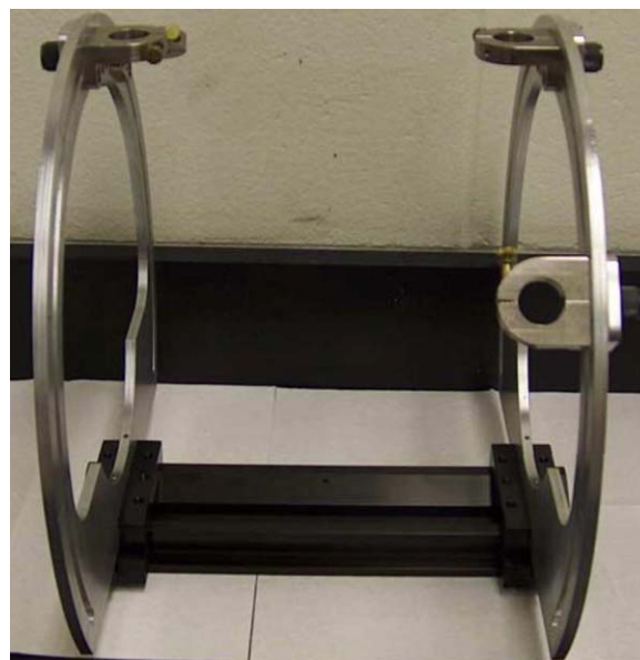
Figure 5. Annular ring assembly to hold the optical probes.
